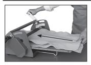
4.1. Turn the handle clockwise while guiding the board through the rollers in the direction of the arrow.
