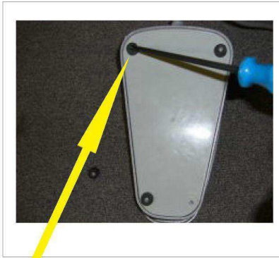
1. Unscrew the 4 feet using the Phillips screwdriver
