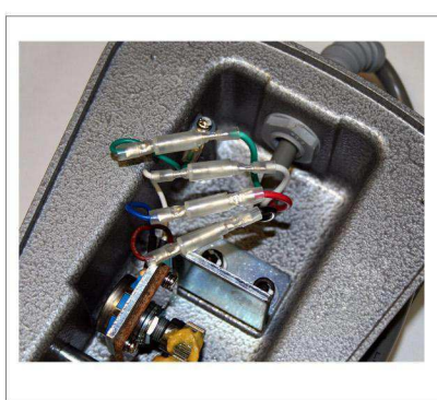
5. Connect the three wires back on to the foot pedal cord: BROWN to BLACK BLUE to RED WHITE to WHITE
