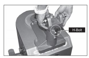
② Mount the Arm Holder on the Jigger Arm Base. Secure Arm Holder to the Jigger Arm Base by tightening the H bolt.
