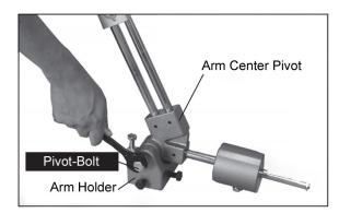
① Remove the pivot bolt on either side of the Arm Holder. Separate the Arm Holder from the Arm Center Pivot. (The Arm Center Pivot is heavy, take care when removing it from the Arm Holder.
