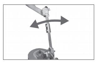
④ Shake the Arm to make sure there is no lateral movement of the Arm Center Pivot in the Arm Holder. If there is movement, tighten the Pivot-Bolts until there is no more lateral movement.
