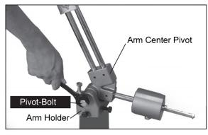
③ Place the Arm Center Pivot into the Arm Holder and secure it by tightening the Pivot-Bolts on both sides.
