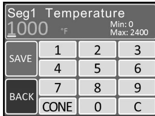
Figure 7: During a Custom Firing, you can enter the desired temperature or press CONE. Choose the desired Cone Number and the controller will enter the corresponding temperature.
