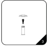
Fix the bottom connection-unit with orientation dowelling.
