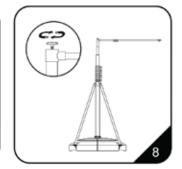
Connect the horizontal-pole and verticalpole with the upper-snail.
