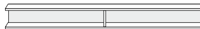
set of 2 shelves with back panel width: 1300 mm, clear height: 124 mm (stabilization against bending)
