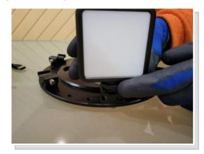
Screw the cylindrical support onto the circular support
