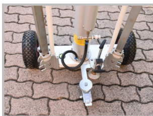
Spherical bubble Releasing air valve Connection for air compressor Kit Security leg with wheel
