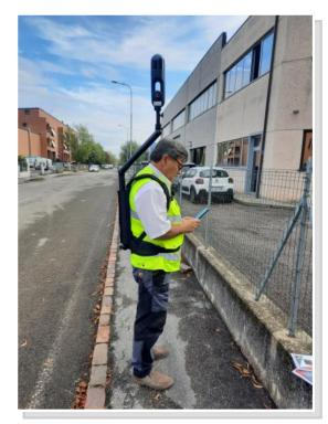
Thanks to the quick release (2) the scanner can be easily used by hand in all situations where the Backpack would be bulky or not suitable
