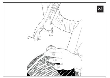
Take the handle and attach it to the cage mounting bracket. The spring loaded button clip locates into the hole in the lower handle.
