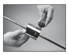
To set the stringing tension, loosen the locking knob on the side of the drop weight. Slide the weight in the appropriate direction until the face *closest* to the string gripper is indexed with the desired tension mark on the tension bar.
