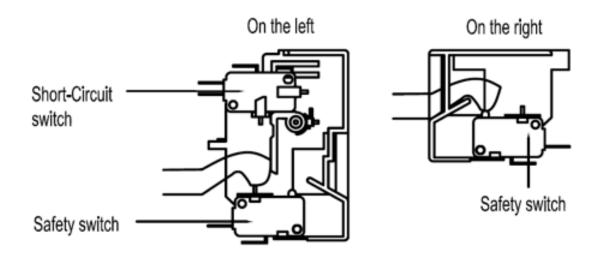
The short-circuit switch works as a safety device in case one of the safety switches doesn't function when required. If the short-circuit switch is activated, it will not be possible to turn the microwave on.
