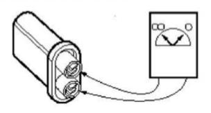
A defective capacitor presents short-circuit (continuity) permanently between its connectors.
