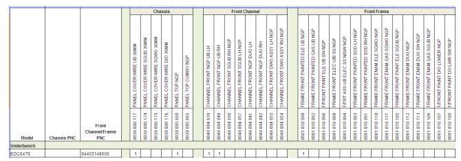
For models with **2** PNC listed the correct parts are all indicated by a number "1" to the right for each applicable change.
