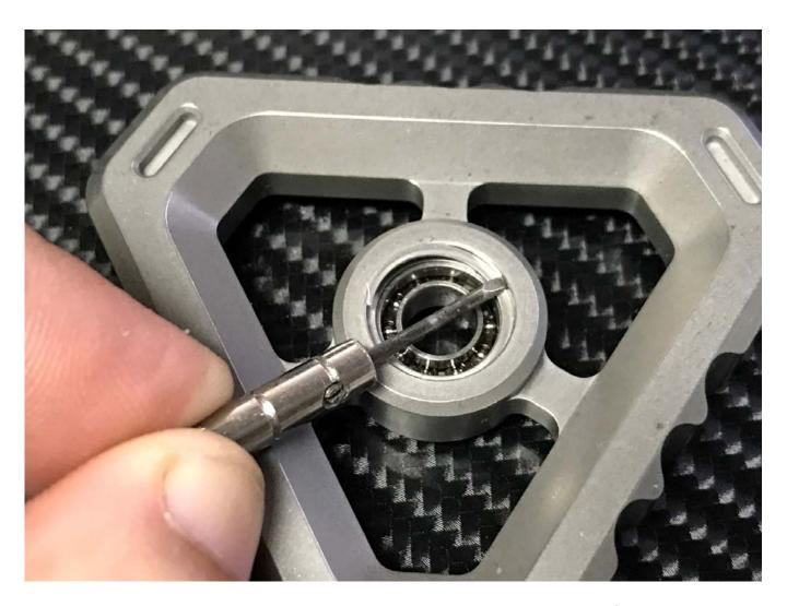
6. Keep pressing the clip around until the whole clip seats inside of the groove. Use the other hand to prevent the clip from springing out.
