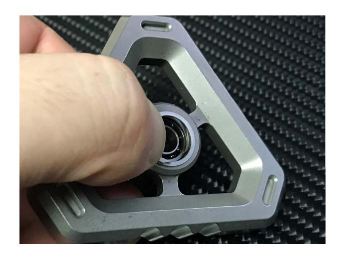
3. Insert the tip of the retaining clip to the retainer groove on the spinner body. Keep pushing it to the groove to prevent it from spring out.
