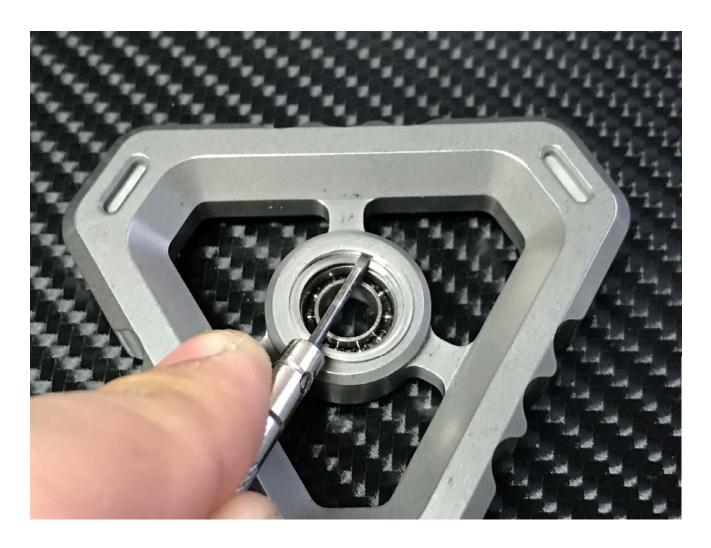
5. Keep pressing the retaining clip down into the groove with the flat head screw driver.
