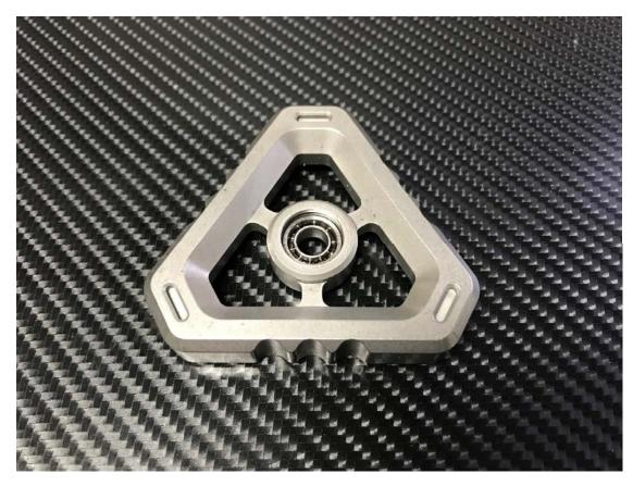
1. Drop the bearing inside of the bearing hole.
