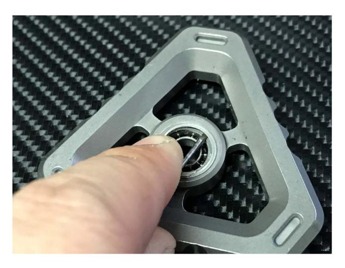
4. Use a small flat head screw driver to press the lower layer of the retaining clip downward to make it seat into the retaining groove. Keep pushing the retaining clip with the other hand to prevent it from spring out.
