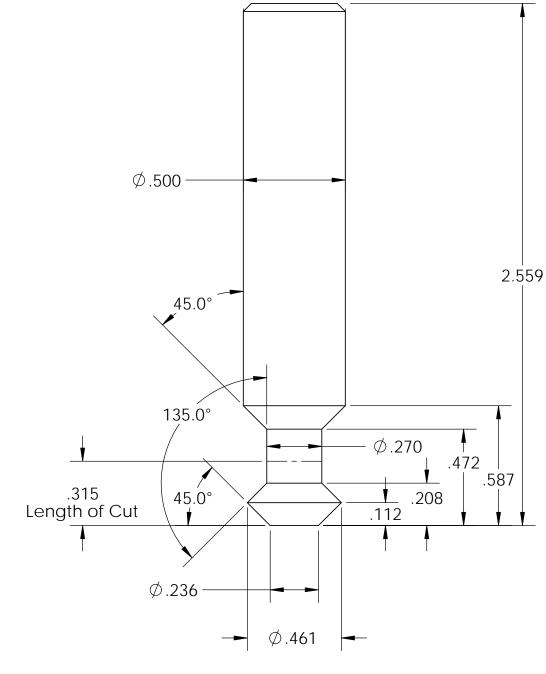
Material: Micrograin Carbide Flute Number: 4 Coating: AlTiN Coated
