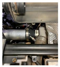
Install the HSM pipe with the welded bungs on it into the 3" boot on the turbo with the hose barbs facing down and the PMAP sensor on the top. Locate one of the 3" rubber loop clamps, the .350 aluminum spacer and the 6mm self tapping bolt. Slide the loop clamp around the pipe. Now put the spacer on the back side of the loop clamp and using a ratchet or driver start the 6mm bolt into the hole on the bedside frame as shown. It may be left just slightly loose for final adjustments.
