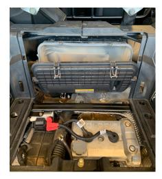
Using pliers twist the pinch clamps until they come apart on the factory blow-off valve hose and breather hose as shown where they connect to the factory plastic intake tube. These clamps will not be re-used, discard them when they break apart. Remove the hoses from the intake tube. Locate factory PMAP sensor in intake pipe and unplug it.
