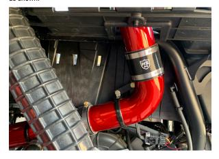
Test fit your air filter onto pipe and make sure the piping is adjusted to desire. Tighten rubber loop by air filter first once desired adjustment is achieved. Working your way toward turbo start tightening all clamps and hardware making sure nothing is hitting or rubbing. Tighten all support brackets to desired adjustments. Double check and make sure all hardware and clamps are tight after all adjustments have been made!
