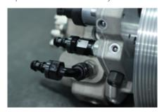
Install the low pressure fuel feed and return lines. Route the 3/8" hose from the 90 degree hose barb fitting on the rear of the fuel filter conversion kit to the straight push-lock fitting at the rear of the CP3 pump. Tighten clamp.
