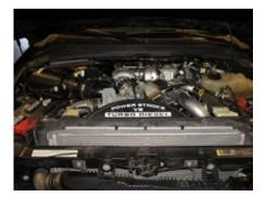
Remove the factory turbo oil feed line assembly. Remove the 4 heat shield bolts from the top of the factory turbochargers and remove the heat shield.
