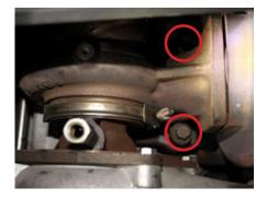
Cover all of the now exposed oil/fuel openings and blow/clean all debris from factory turbo pedestal area. Remove the factory oil drain tube from the driver side of the factory pedestal.
