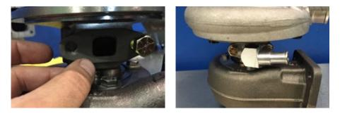
Locate the supplied T4 exhaust flange gasket and four 3/8" flange nuts. Install the turbocharger onto the HSM cast pedestal/elbow in the vehicle and tighten the nuts to 30 ft-lbs. Torque the exhaust up-pipe bolts to 25 ft-lbs before torquing the pedestal/elbow support plate bolts to 45 ft-lbs.
