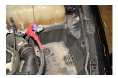
Remove the 2 coolant lines from fuel cooler assembly and remove the fuel line banjo bolts from the top side of the fuel cooler assembly.
