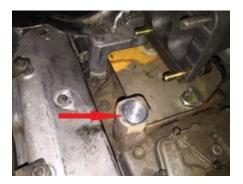
Locate the supplied oil feed adapter, adapter hold down, black o-ring, and -6an to 1/8" NPT oil feed fitting. Slide the hold-down over the adapter and using pipe thread sealant, install the fitting into the adapter. Apply some grease/lube to the o-ring before installing it onto the adapter and then installing the adapter assembly into the oil supply hole in the oil cooler. Install the previously removed factory bolt and torque to 12 ft-lbs.
