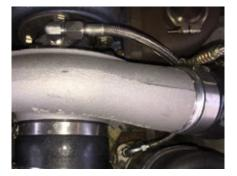
If you will not be using an external wastegate, block the wastegate port on the cast elbow using the supplied plug and clamp.
