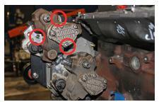
Locate the supplied dual fuel pump pulley, pulley retaining nut, and lock washer. Install the pulley onto the CP3 pump using the supplied hardware. Carefully hold the pulley in place by using the holes machined in the pulley or by using another pulley holding tool and torque the nut to 75 ft-lbs.
