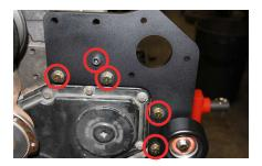
Locate the supplied angle support bracket, (2) 3/8x16x1.25 bolts, (4) 3/8 flat washers, (2) 3/8 nyloc nuts, and (2) M10x1.5x20mm flange head bolts. Loosely install the angle support bracket to the main pump mounting plate and cylinder head as shown (the M10 bolts will be used for the cylinder head side). Torque all (6) 3/8 mounting plate hardware to 35 ft-lbs first, torque the front 8mm socket head bolt to 25 ft-lbs, and torque the (2) 10mm bolts on the cylinder head last to 35 ft-lbs.
