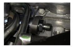
Put the supplied high pressure fuel distribution block into a vise and install the factory fuel rail pressure sensor into the sensor port on the block. Torque the sensor to 70 ft-lbs.
