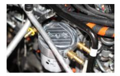
**NOTE:** Push-lock fittings do not require hose clamps. Put a dab of clean engine oil on the hose barb end and firmly the push hose onto barb until it is fully seated.
