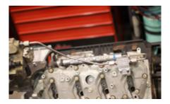
Locate the factory CP4 pump wire harness. Disconnect the harness from the factory CP4 pump and install the supplied wiring harness as shown. Route the supplied harness away from hot/moving parts and connect the other end to the HSM CP3 pump.
