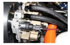
Route the two supplied 1/2" lines to the factory fuel supply as shown. Tighten clamps.
