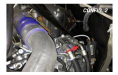
Install the supplied fuel "T" fitting and plumb the return fuel system as shown. Route the HSM CP3 pump return line from the 90 degree push-lock on the top of the CP3 pump to one side of the "T". Use the supplied 3/8" hose to connect the "T" back to the factory return line. On "Config 2" fuel system equipped vehicles, you will need to use the supplied quick-connect fitting to connect the supplied fuel line to the factory return line.
