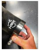
**Note:** Make sure when installing the clamp on the intercooler end of all boots to be sure the clamp is pushed up close against the intercooler outlet as shown, so the intercooler outlet does not cut the boot if the clamp is tightened too far out.
