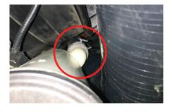
Reconnect the factory intake air temperature sensor connector and clip/zip-tie the wiring harness away from any hot/moving engine components. Reconnect vehicle batteries and double-check all work.
