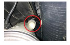
silicone hose. Reconnect the factory intake air temperature sensor connector and clip/zip-tie the wiring harness away from any hot/moving engine components. Reconnect vehicle batteries and double-check all work.
