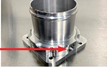
Install the previously removed throttle valve gasket onto the supplied HSM throttle body adapter (it will only fit one way). Use the supplied  $6 \text{mm} \times 1.0 \times 20 \text{mm}$  allen head bolts to hold the gasket to the HSM throttle body adapter (as shown) while you install the HSM throttle body adapter to the factory intake manifold assembly. Torque all 4 bolts to 98 in-lbs.
