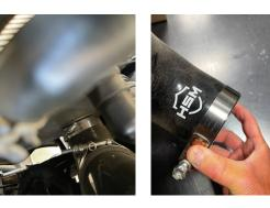
**Note:** Make sure when installing the clamp on the intercooler end of all boots to be sure the clamp is pushed up close against the intercooler outlet as shown, so the intercooler outlet does not cut the boot if the clamp is tightened too far out.
