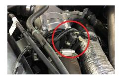
With a pick tool or something similar, carefully remove the metal locking clip from the factory plastic throttle body coupler as shown. Pull the coupler off of the factory throttle valve assembly as shown.
