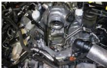
Remove the two bolts holding the metal coolant pipe to the engine and carefully slide it out of the aluminum thermostat housing to remove it. Set the coolant pipe and hardware aside for re-use later.
