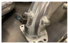
Apply a small amount of assembly grease or clean engine oil to the O-ring on the previously removed OEM metal coolant pipe and re-install it in the factory location. Securely fasten the pipe using the OEM hardware and reconnect the plastic locking connection on the OEM coolant hose.
