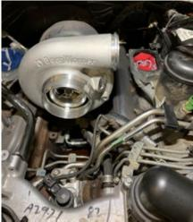
Using glass cleaner on the silicon boots, install the HSM hot side intercooler pipe using straight 3" boot on the intercooler and the straight 3" boot on the turbo compressor outlet as shown. Adjust and tighten all clamps.
