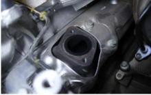
NOTE: The clearance between the driver side manifold and the fuel lines can be tight, be extremely careful not to apply excessive pressure to these fuel lines while disconnecting the hardware or removing the manifold.
