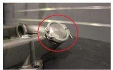
If some of the exhaust manifold studs were pulled out of cylinder heads during the removal of the OEM exhaust manifolds, carefully remove the nuts from the studs and re-install the studs into the cylinder heads now. Ensure they bottom out correctly into the cylinder heads but DO NOT over-tighten as the cylinder heads are aluminum.
