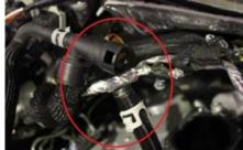
NOTE: Removing the hot-side intercooler pipe first can also free up some extra space for the plastic intake manifold removal if necessary.
