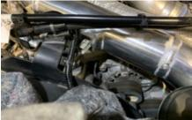
NOTE: We recommended using glass cleaner on all boot connections for ease of install and a clean connection surface.
