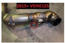
**NOTE**: On some vehicles, it may be easier to access the v-band clamp through the passenger fender-well.
