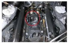
NOTE: A short 9/16" wrench will be the easiest way to tighten the driver side mounting nuts as they are a very tight fit. The passenger side nuts can be easily reached with a ratchet and extension.
