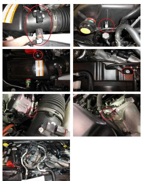
Remove the bolt holding the engine and transmission oil dipstick tubes to the plastic intake manifold and unplug the MAP sensor electrical connection on top of the plastic intake manifold. Un-clip any electrical harnesses or coolant hoses that are attached to the plastic intake manifold.
