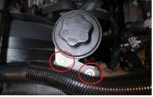
Remove the charge air temperature sensor from the OEM intercooler piping by carefully disengage small locking tab while twisting the sensor counter-clockwise. Clean the sensor of any oil/debris and install it into the supplied HSM cold-side intercooler pipe with a small amount of assembly grease or clean engine oil on the O-ring to aid in installation and prevent damage. Ensure the sensor is fully locked into place as shown.
