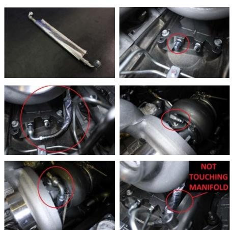
Using the supplied 3/8" hose clamp, install the supplied coolant hose between the pedestal coolant fitting (driver side fitting) and factory thermostat housing as shown. If you are using an EGT solution, install the previously removed EGT sensor into the appropriate port on the driver side exhaust manifold and plug in the EGT sensor electrical connection.
