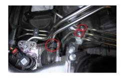
On early 2011 model year vehicles, sometimes there is a stud protruding from the firewall that must be trimmed for downpipe clearance. Using a grinder or saw, carefully trim approximately 1/2" from this stud. Slide the supplied HSM upper downpipe section into its approximate location from the top. It will be connected at a later time.
