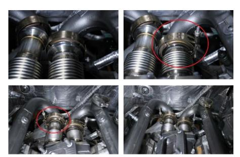
Ensure that the manifold and pedestal assembly are aligned correctly and no potential exhaust leaks or other issues can be found. Torque the exhaust manifold mounting hardware to 25 lb/ft.
