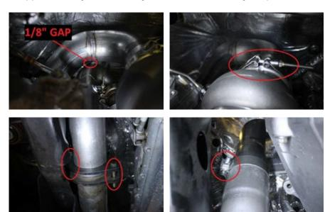
fitting (passenger side fitting, marked "0" for OIL) and turbo oil feed fitting on top of the turbocharger center section. Route the oil feed line in a manner so that it does not interfere with any other parts and is away from heat as shown. Double check that the oil feed line is connected to the correct PASSENGER SIDE fitting on the HSM pedestal! Connecting it to the incorrect port will almost certainly result in turbocharger damage and possibly other engine damage!
