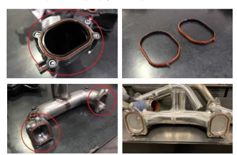
NOTE: The clearance between the turbo compressor housing and firewall is tight. The easiest method to install the intake manifold is by sliding the driver side in first, then work the passenger side between the turbo and firewall.
