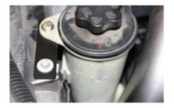
Zip-tie the intake air temperature wiring to the nearby coolant line as shown. Reconnect batteries and double-check all installed items for proper fitment. Test drive vehicle to ensure all parts were installed correctly.
