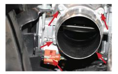
Release the factory intake air temperature sensor locking tab and twist the sensor to remove it from the factory intercooler pipe. Install the previously removed sensor into the supplied HSM throttle body assembly.
