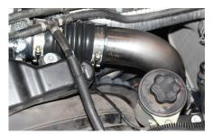
Reconnect the factory intake air temperature sensor. Drill a small hole in the top of the factory fan shroud and zip tie the intake air temperature sensor wiring harness to secure. The factory clip on the wiring harness may be reinstalled into lower hole in the fan shroud.
