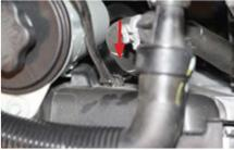
Remove the t-bolt clamp at the factory intercooler connection. Remove the factory power steering reservoir bolt from the fan shroud and set aside.
