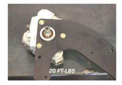
Gather the supplied hardware for the pump/bracket installation - (3) M8x1.25x150mm bolts, (3) flat washers, and (1) lateral support spacer. One of the factory fan hub bolts will be re-used with the lateral support spacer.
