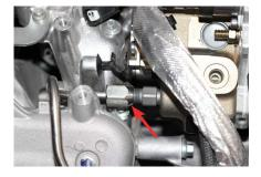
Install the (3) supplied M8x1.25x150mm bolts into the pump bracket and tighten evenly while supporting weight of pump to ensure no binding occurs. Torque bolts to **20 ft-lbs**.
