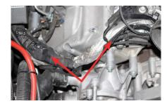
Locate and unplug the factory CP4 wire harness connector. Re-route the harness toward the front of the engine, exposing the connector for easy access. Remove the gray locking sleeve from the connector. The outer tabs of this sleeve must be shaved/removed as shown in order to connect it to the new supplied harness. After modifying, re-install the gray locking sleeve to factory connector.
