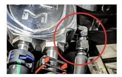
NOTE: Push-lock fittings do not require hose clamps. Apply a dab of oil on hose barb end and carefully push hose on to the barb. Route the fuel lines away from heat or any places where the lines may rub. Fuel line routing may vary due to different fueling and turbo setups.
