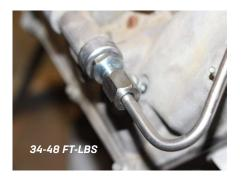
Install the supplied high pressure fuel line support on factory valve cover stud as shown.
