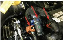
After all fuel lines are disconnected from the factory fuel filter, carefully twist the filter counter-clockwise to release it from the factory filter mount as shown. Carefully pull up and remove the factory fuel filter from the vehicle. The factory fuel filter assembly can be discarded at this time.
