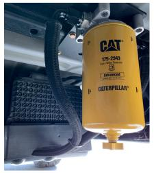
Turn the key to the run position for 30 seconds and prime the system. Do not start the engine! Repeat this process until the system is primed, this may take 4-5 key cycles. Start engine and check for proper function of system. You may notice some noise from the factory fuel pump while the air is purged out of the system. This is normal.
