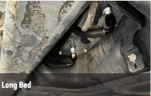
Locate provided CAT filter. IT HAS A PROVIDED O-RING WITH IT THAT MUST BE INSTALLED ON THE FILTER POST AS SHOWN!!!!!! This will ensure proper function of the filter and system. Lube the fuel filter o-ring and install the fuel filter onto the housing. Hand tighten.
