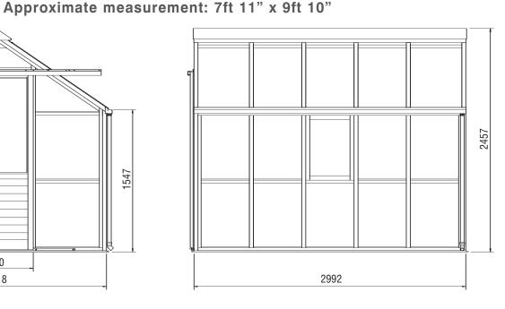
The framework and cladding is in a top grade Western Red Cedar which is grown on the Western Sea Board of North America. It has long been used in inclement climates in the construction and garden industries due to its longevity (the timber contains natural preservatives), stability (it does not easily warp or bend being straight grained) and strength. All of our cedar is sourced from certified or sustainable forests.
