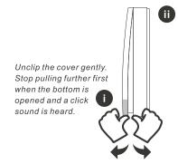
Continue to pull the bell push cover open slowly and carefully to unfasten the upper corners of the cover from the joints. If the cover is locked too tight by the joints, try to sway the cover slightly to loosen it up.
