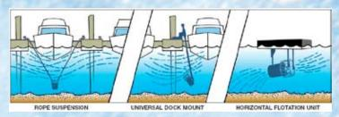
**ROPE SUSPENSION:** Use ropes or cables to suspend unit in vertical or angled position.
