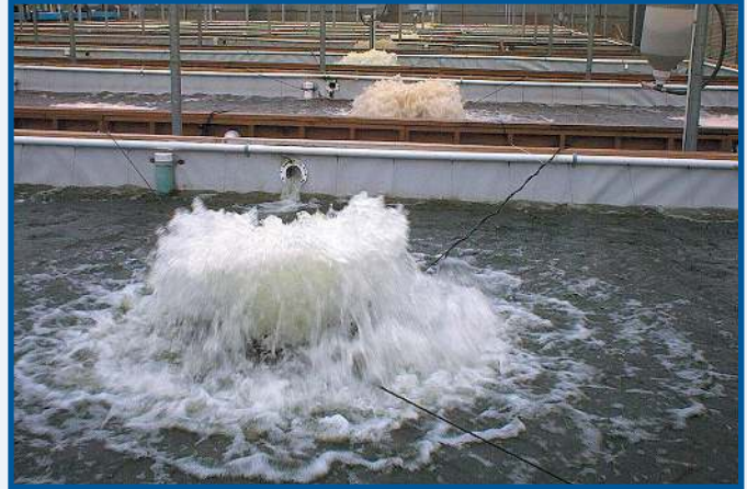
TANKS: This Tilapia farm uses Kasco Aerators to maintain densities of up to .4 lbs of fish per gallon of water. The aerators are also used to vent carbon dioxide.
