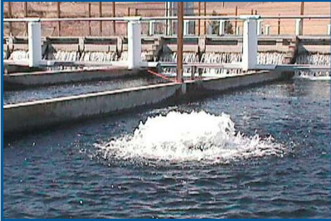
RACEWAYS: Kasco Aerators can be used to increase oxygen levels during feeding, as well as to increase fish densities.
