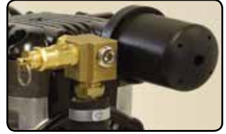
Figure 1. Note the compressor intake and outlet when installing air filter and outlet assembly.
