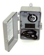
Optional UL Approved Control Panel complete with Class A Human Rated GFCI Protection, 24 Hour Mechanical Timer, and Photo Eye for Optional Light Kit. NEMA Type 3R weatherproof enclosure.
