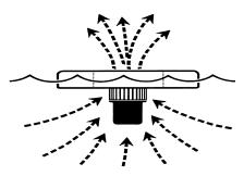
During unit operation, water is circulated from  $360^{\circ}$  around the unit as well as from below. Top intake for shallow water operation.
