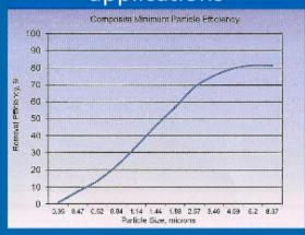
The efficiency chart above is extrapolated from particle size Versus efficiency information when evaluated per ASHRAF Standard 52.2
