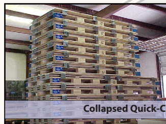
Strength Test - 9000 lbs of load
