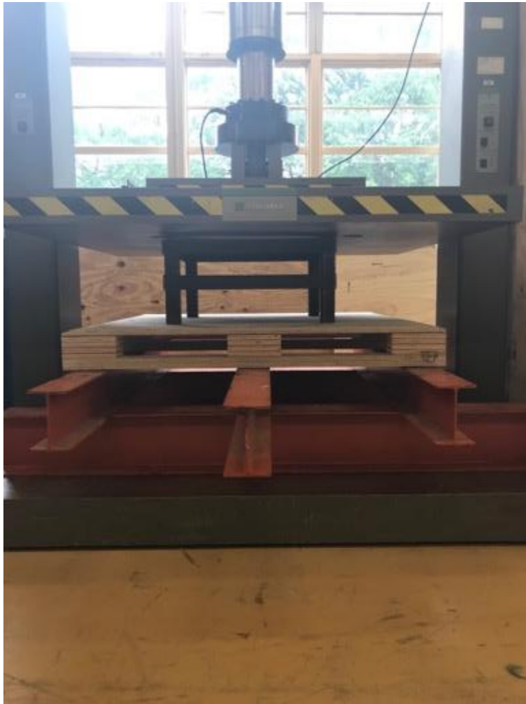
Figure 5: Crate Base with Metal Fixture on Interlaken Compression Tester
