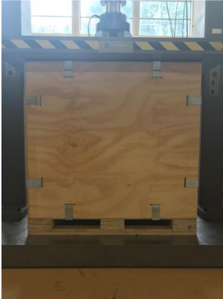
Figure 1: Crate on Interlaken Compression Tester
