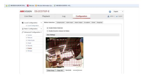
Click 'Edit' to set the time table of motion detection (e.g. 24h/7 days). Time table will show blue if you have set. Click 'Trigger Channel' in linkage method to set it trigger recording. See following:
