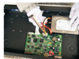
2.HDD data line and power line connection
