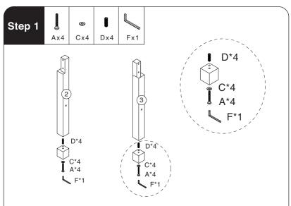
Please identify which leg is ② and which leg is ③ according to the drawings. You can easily add the 4 extender blocks to the legs to adjust the height. If your Lego table does not need to increase in height, please skip this step.
