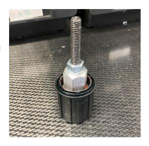
Once the expanding collet is gripping the bearing securely, the 'cup' is placed over the expanding collet, followed by the outer washer and nut. Ensure the cup is centred.
