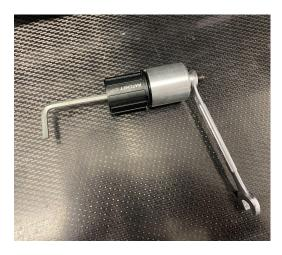
4 Afterwards, to remove the bearing from the extractor, remove the outer nut and cup and then undo the inner nut on the collet a few turns.
