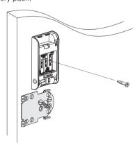
Fix screw to completely secure battery pack.
