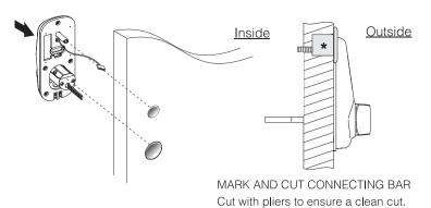
Place the Electronic Keypad into the holes on the outside of the door. Following the Mounting Instructions provided with your Deadlatch, measure and cut the connecting bar to the required length.
