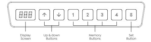
The whole handset surface is a button panel. If there is no press within 30 seconds, the screen is locked and 1/2/3/4/S keys are locked correspondingly, press the Up or Down buttons first, handset can then be used when the display screen lights up.
