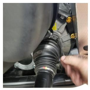
**14.** Pull axle out: position axle parallel with the ground and pull by gripping the outer CV housing and axle shaft.
