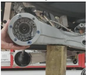
**18.** Measure from outer face of transaxle hole to outer face of trailing arm hole. Measurement should be:
