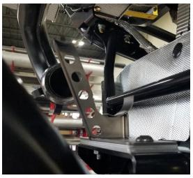
10. Place exhaust on mount and fit intake bell to the exhaust ball flange. Make sure to orient it correctly, as shown below.
