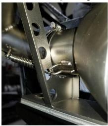
11. There is extra clearance between the mounting bolts and the frame holes to allow the mount to be adjusted left-right and front-back. Move the mount until the exhaust is sitting tight into it and there is clearance between the exhaust and the vehicle.
