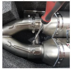
**8.** Remove hardware from exhaust mounting bracket/shims.
