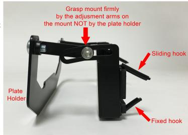
**Step 2:** With the mount in place take the included hex tool and loosen the screws on either side of the front plate mount. With the screws loose slide the plate mount forwards or backwards as needed to get the plate clearance and angle desired. When the final position is achieved, firmly tighten the Allen head (hex) bolts.
